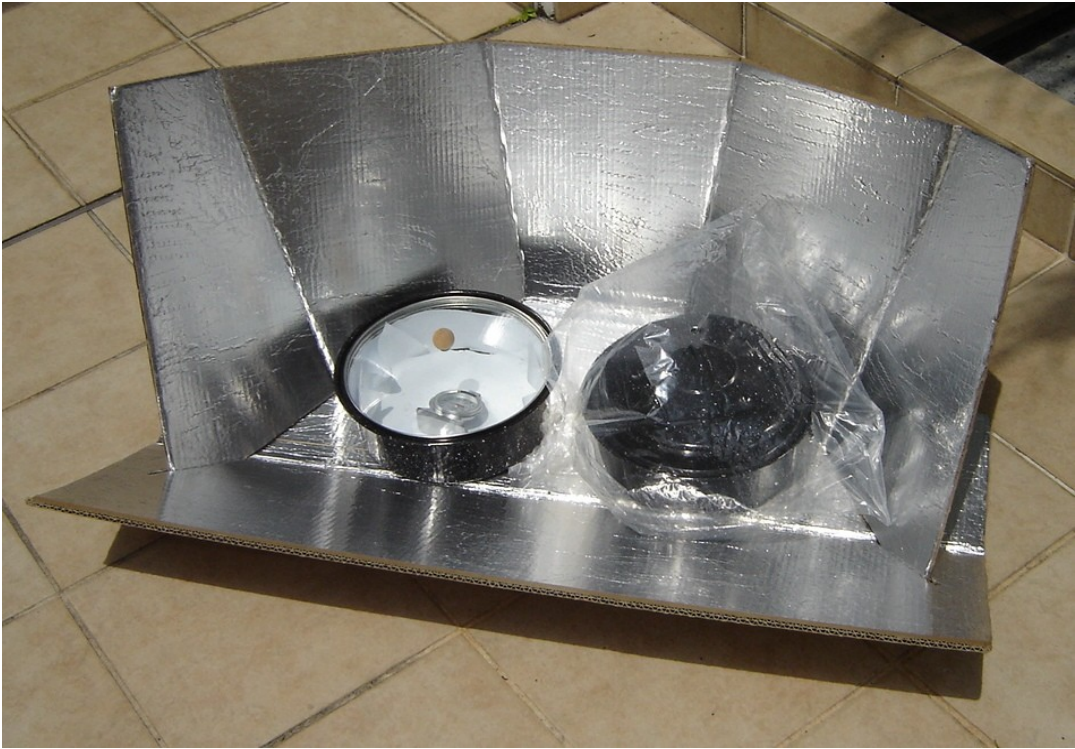
'CookKit' containing a pot with a clear glass lid next to a pot with a metal lid and enclosed in an oven bag
